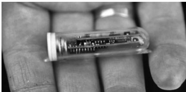
Figure 8. A mini Conductivity-Temperature-Depth (CTD) archival tag (Data Storage Tag, Star-Oddi Marine Device Manufacturing, Reykjavik, Iceland). Reproduced with permission from Star-Oddi.
