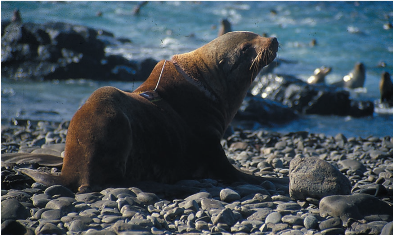
Plate 132. A Time-Depth Recorder (TDR) and Platform Transmitter Terminal (PTT) attached to a male fur seal Photograph R. Kirkwood.
